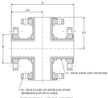
BODY MATERIAL: AISI 1010 - 1030 STEEL ASTM A516 GRADE 70 ASTM A105
