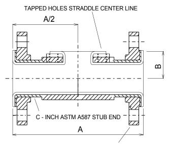
D - INCH CLASS 150 ASTM A105 STEEL MODIFIED SLIP ON FLANGE
