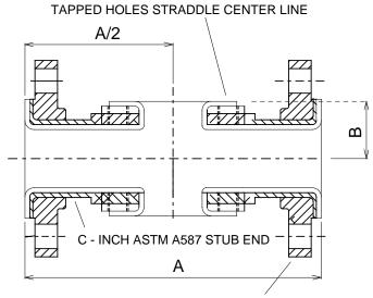
D - INCH CLASS 150 ASTM A105 STEEL MODIFIED SLIP ON FLANGE
